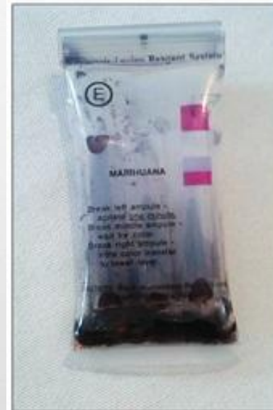
The NIK Duquenois-Levine rendering a false positive after testing a chocolate bar.
