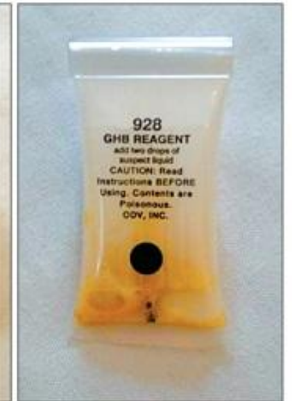
The NarcoPouch 928 GHB Reagent Test rendering a negative result.
